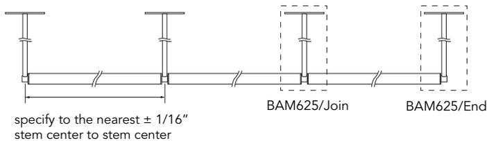
Two BAM625/End required for each fixture run
