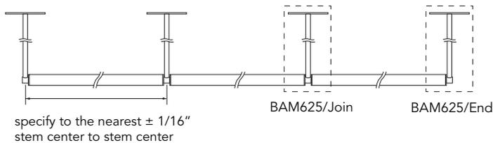
Two BAM625/End required for each fixture run
