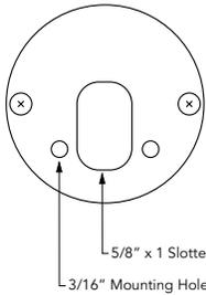
**EC922** Pair end caps w/ drop mounting holes (for wood end case mounting)
